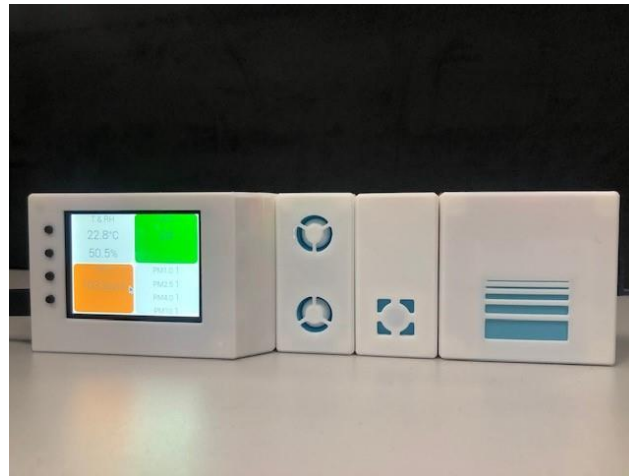
Figure 17: RS DesignSpark Air Quality kit
